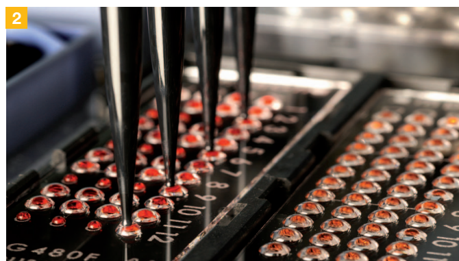
Automation of 1 \mu l AmpliGrid AG480F amplification reaction on Hamilton MICROLAB STAR LET , SW version 4.1
