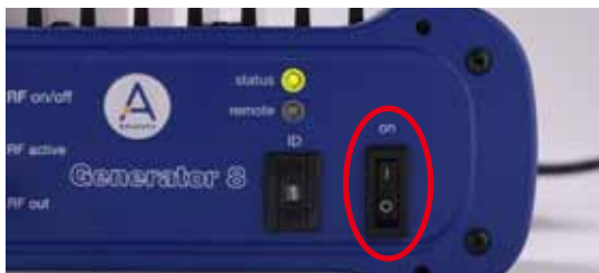
Figure 5: Generator8 front panel controls
