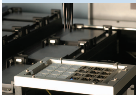
mixing unit mounted in pipetting robot
